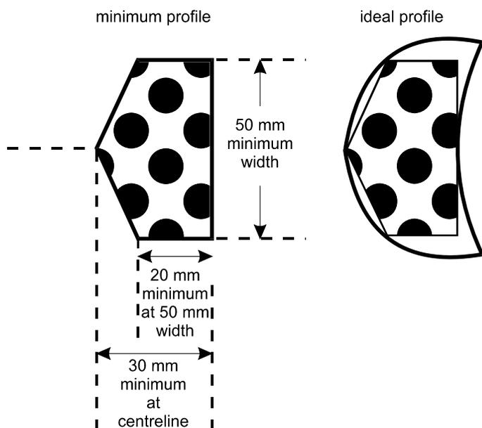
1.4. The padding must be positioned on the edge (see definition of edge in kayak specifications) to cover at least 15 mm above and below the edge.
