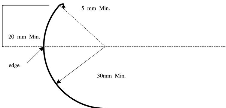
12.5. Recesses in the hull or deck for the purpose of hiding bolt or screw heads etc. are to be permitted. Recesses should be safer than a projecting fixing device in order to be legal. Where recesses are provided to improve safety by eliminating projecting fixing devices, the 5mm radius shall be relaxed as far
