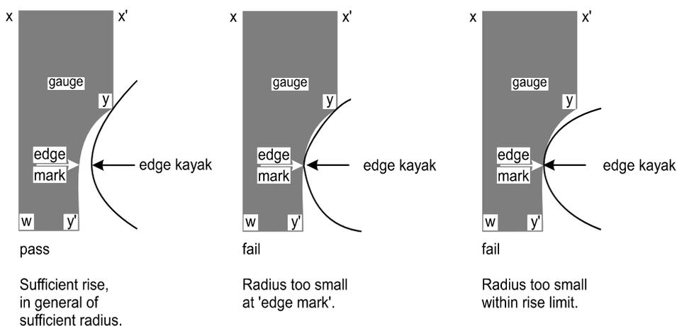
3. To gauge the radius of curvature the radius portion of the appropriate gauge, must be applied perpendicular to the surface being tested. If both points X and X' touch the surface at the same time without the rest of the kayak, the test is passed.
